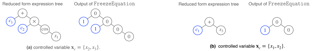
Figure E.1. Visualization of the FreezeEquation function. 0 implies the node is non-editable and 1 implies the node is editable, by the GP algorithm. The FreezeEquation function will increase the probability of finding expression trees with close-to-zero fitness scores.
